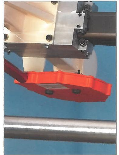
Every CollinsCraft Roll Slitter is supplied with two blade canisters. Roll rotation is reversible which extends the life of our proprietary blade. Empty canisters returned for refill are processed and shipped back the same day.
