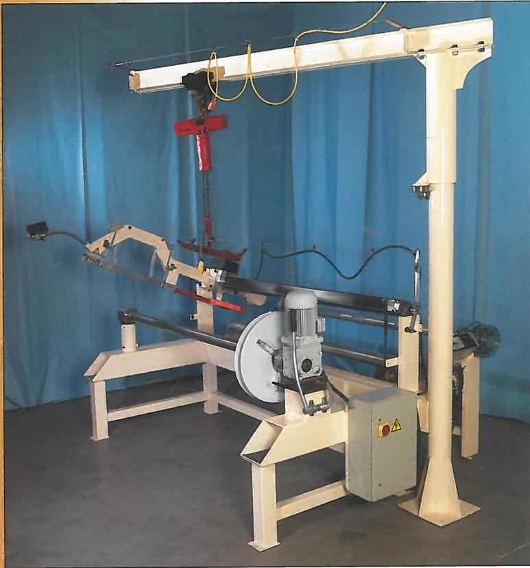
CollinsCraft Roll Slitter Model 76-24 with jib crane hoist and re-roller attachments pictured are offered as options.
