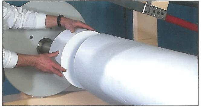
Every cut is neat, clean and to the exact measurement. Blade life is lengthened because it stops short of the non-rotating mandrel.
