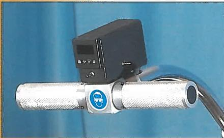
Cut widths may be programmed in either metric or English measurements. Slitter controls are easy to use and within reach of the operator. The standard slitter is manually positioned to the cut width. Options include Auto-stop and Auto-index.
