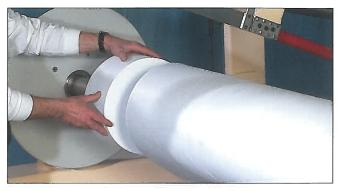
Every cut is neat, clean and to the exact measurement. Blade life is lengthened because it stops short of the non-rotating mandrel.
